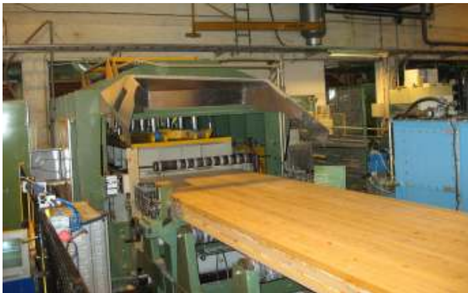
Figure 22 Radio-frequency press for cross-laminated panel
