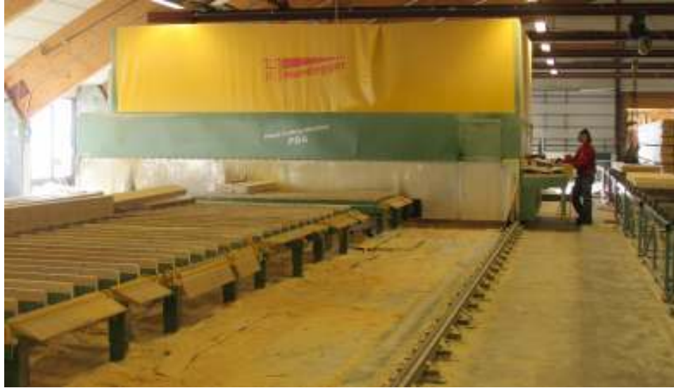
Figure 23 CNC Machine – PBA from Hundegger
