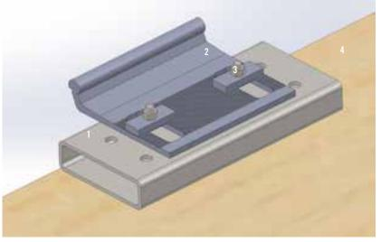
HSS 178 x 51 x 6.4 screwed to NLT panel. Concrete overpour flush to top of HSS.
